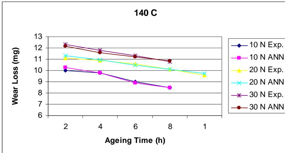
**Figure 9.** The comparison of experimental wear loss values with ANNs results of 6063 Al alloy at 140 °C ageing temperature and different applied loads.
