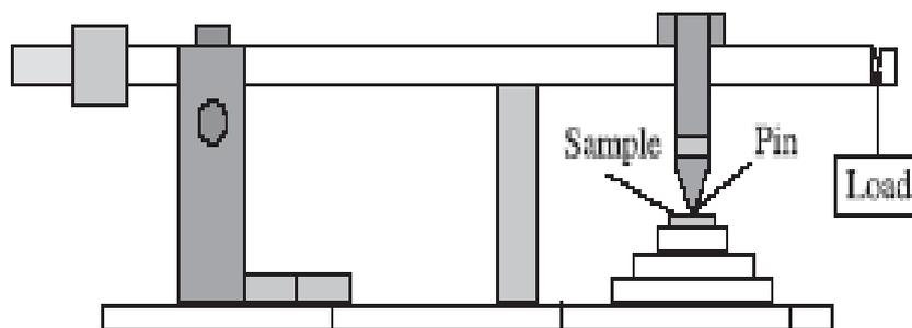
**Figure 2.** Schematic representation of the pin-on-disc test configuration [Gavgali et al].
