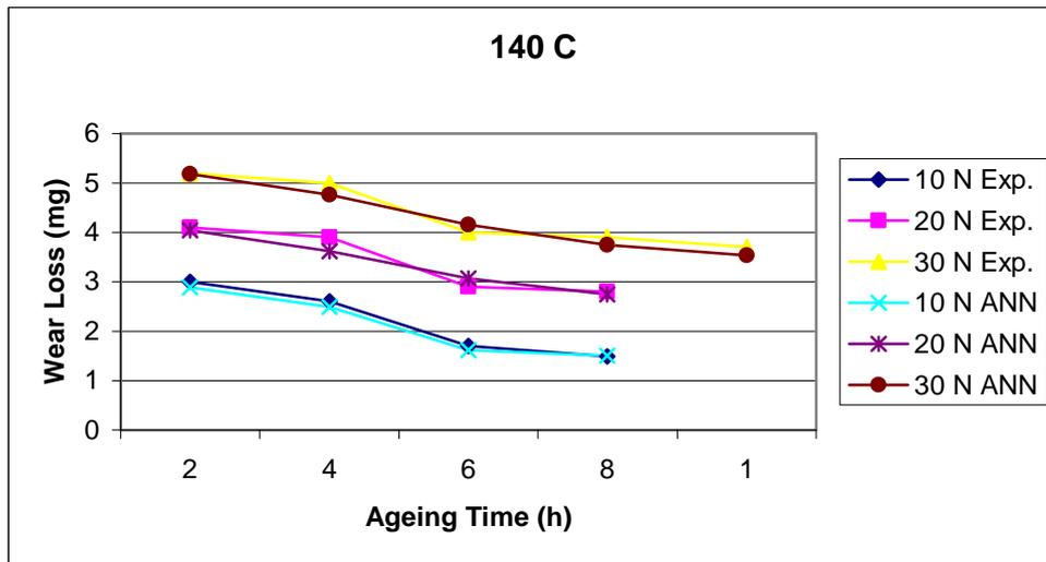
**Figure 5.** The comparison of experimental wear loss values with ANNs results of 2024 Al alloy at 140 °C ageing temperature and different applied loads.
