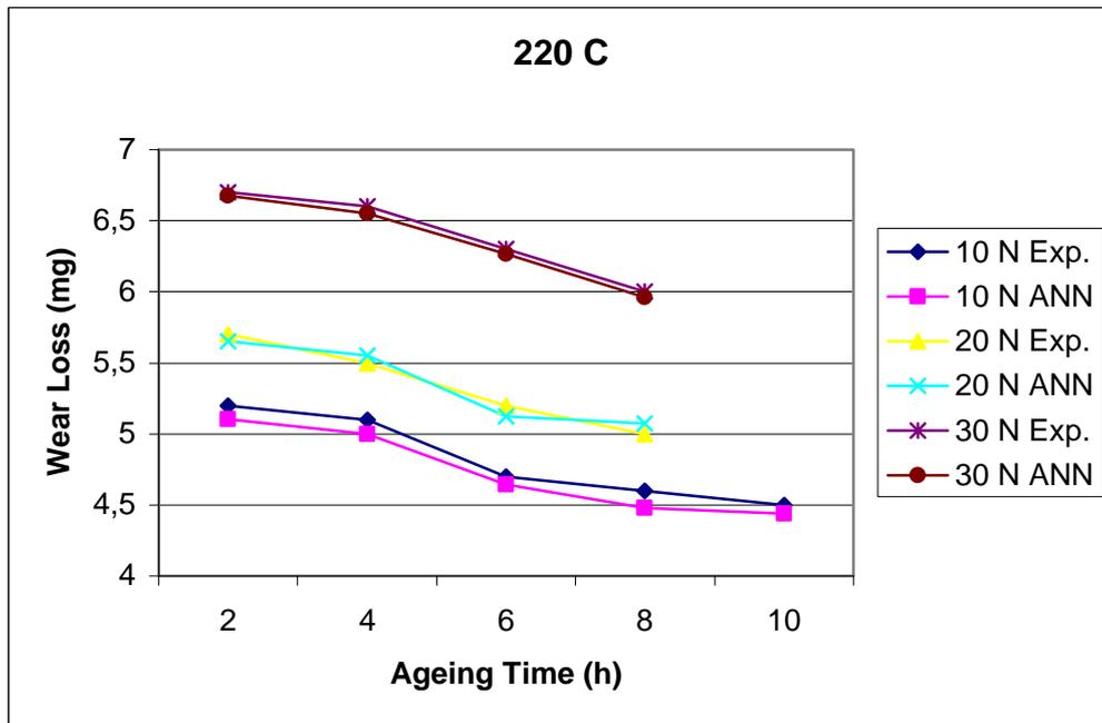
**Figure 7.** The comparison of experimental wear loss values with ANNs results of 2024 Al alloy at 220 °C ageing temperature and different applied loads.
