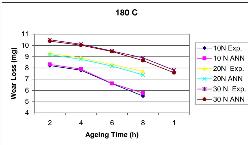
**Figure 10.** The comparison of experimental wear loss values with ANNs results of 6063 Al alloy at 180 °C ageing temperature and different applied loads.
