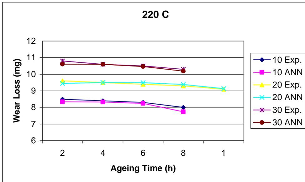
**Figure 11.** The comparison of experimental wear loss values with ANNs results of 6063 Al alloy at 220 °C ageing temperature and different applied loads.
