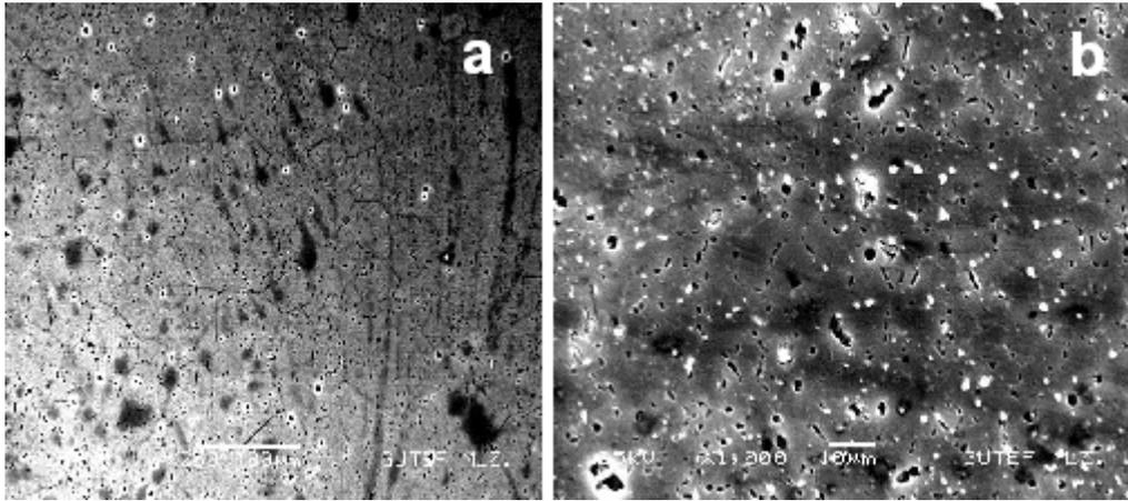
**Figure 3.** SEM images of the AA 6063 and AA 2024: (a) at 140 °C aged for 10 h of AA 6063; (b) at 180 °C aged for 2 h of AA 2024.
