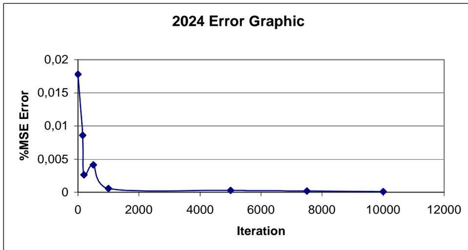
**Figure 4.** Iteration number versus mean square error for training nonlinear correction coefficient for aged 2024 Al alloy.
