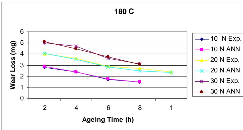
**Figure 6.** The comparison of experimental wear loss values with ANNs results of 2024 Al alloy at 180 °C ageing temperature and different applied loads.
